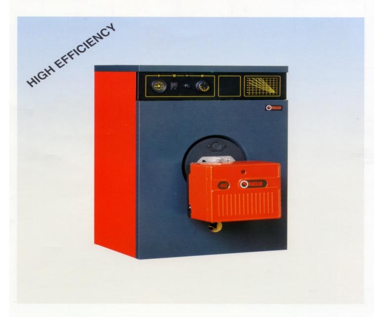
There are 8 models of the 2 RCT range of boilers with rates from 27 kW (92,124 Btu/hr) to 97,2 kWn (331,646 Btu/hr). The cast iron heat exchanger incorporates 3 flue passes to ensure maximum heat transfer and the boilers are comprehensively insulated with a special material in order to minimise heat loss and to reduce combustion noises.
